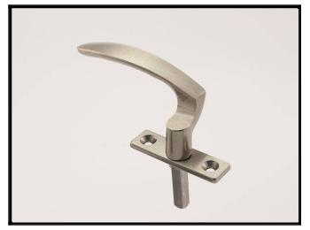
Melron bronze architectural hardware is handcrafted from start to finish in our Central Wisconsin facility. The product you choose is cast in a sand mold, tumbled, machined and finished by our small group of skilled craftspeople. The texture of the sand grains used to make the mold give our hardware its unique characteristics.
